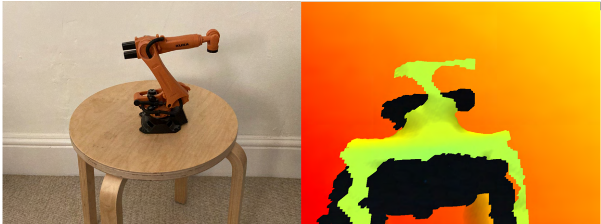
Figure 2.8: Example of photogrammetry. Left shows a RGB image of a model robotic arm. Right shows a depth camera interpretation of the same scene.
