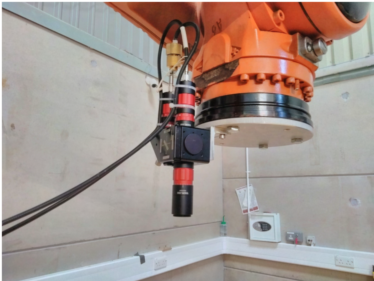
Figure 7.9: Stand-off Raman probe attached to KUKA KR150.
