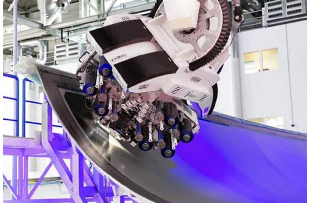
The MTorres automated fibre placement head at Airbus applying composite tape to an A350 wing cover tool
