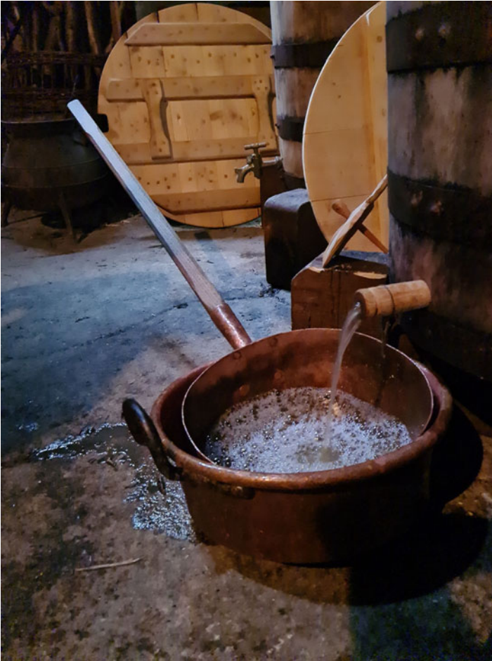
Figure 9. Wort running through the wilch and tube tap into the ladle.
