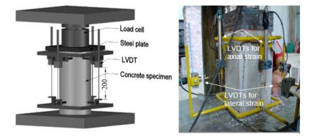
Figure 4. Test setup and position of LVDTs for axial and lateral strain measurements.
