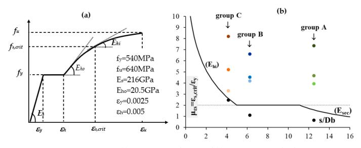
**Figure 8.** (a) Bar stress–strain diagram and (b) compressive strain ductility,  $\mu_{\epsilon s}$ , versus stirrup spacing s/D<sub>b</sub> for the longitudinal reinforcement used in the tests (dots refer to experimental values of  $\mu = \varepsilon_{ccu} / \varepsilon_{v}$ ).
