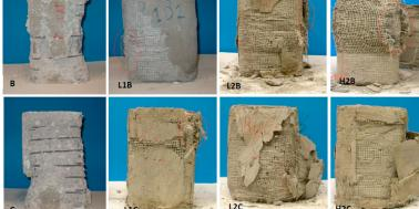
Figure 5. Control (X = A, B, C) and SRG-jacketed columns (DiX) at failure.
