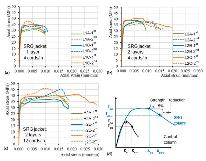
**Figure 7.** Axial stress–strain curves of the tested SRG jacketed columns; (**a**) 1 layer–4 cords/in; (**b**) 2 layers–4 cords/in; (**c**) 2 layers–12 cords/in. (**d**) Nomenclature for the axial stress–strain milestone points.
