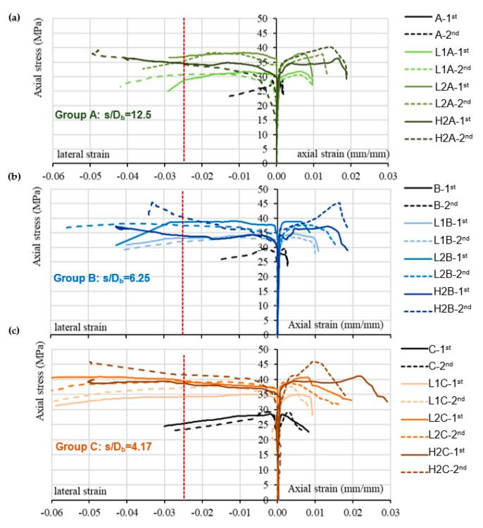
**Figure 6.** Axial stress-axial/lateral strain curves of the tested columns of (**a**) group A ( $s/D_b = 12.5$ ); (**b**) group B ( $s/D_b = 6.25$ ); (**c**) group C ( $s/D_b = 4.17$ ).
