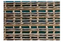
Figure 2. Unidirectional ultra-high strength steel textile.
