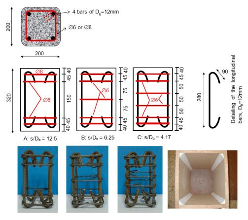
**Figure 1.** Geometry and reinforcement detailing of the columns (dimensions in mm), steel cages of the three groups of specimens and mould with rounded corners.
