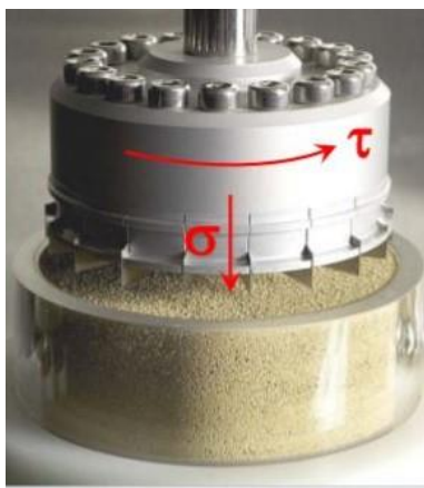
Figure 9 An image of the shear cell loaded in the FT4 to determine the shear flow of consolidated powder.
