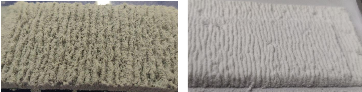
Figure 12. Deposition trial using PA12 combined with 30% milled carbon fibre (left) and unmodified PA12 (right)
