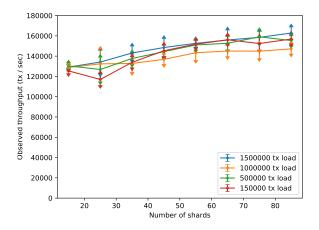
Figure 11: Variation of the throughput of transfer orders with the number of shards, for various loads. The in-flight parameter is set to 1,000.
