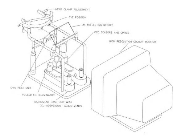
Figure 2.1 Schematic drawing of the P\_SCAN 100 system for the simultaneous measurements of pupil diameter and 2-D eye movements. The diagram shows the instrument base unit which allows easy adjustment of the CCD sensors as required for positioning and focusing of the images of the eyes, and the high resolution colour monitor which is used for generating the visual stimuli
