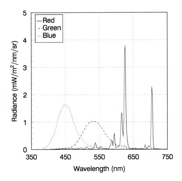
Figure 2.4 Spectral radiance of the three phosphors of the screen used in the experiments described in Chapters 3, 4 and 5
