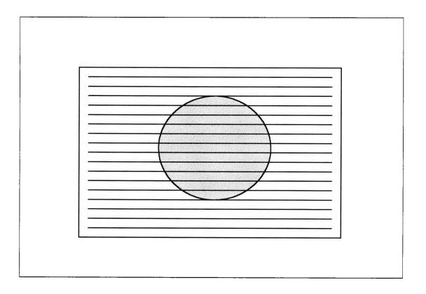
Figure 2.2 Diagram to illustrate appearance of pupil and scan lines in the P\_SCAN 100 system. The co-ordinates of the points of intersection of the scan lines and the pupil margin are extracted by the hardware every 20 ms. The best circle is fitted to the co-ordinates measured, and its diameter and centre position are calculated for each frame.
