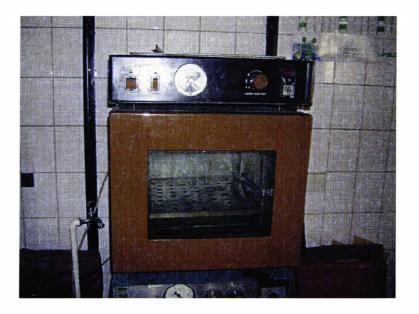
Figure 3.5 Vacuum drier used for the experiments
