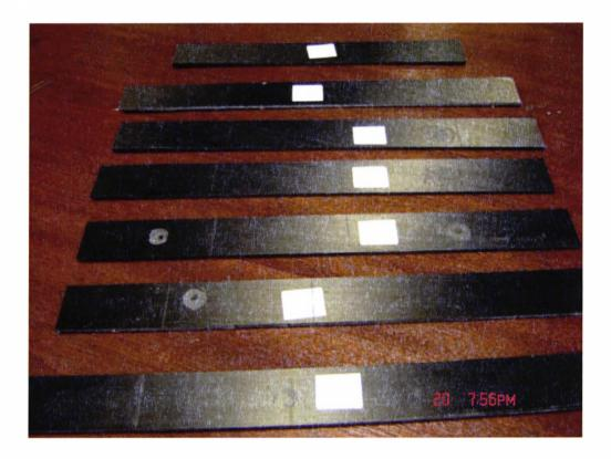
Figure 9.10 Tested composite beams
