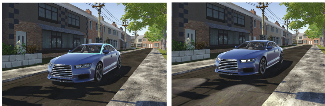
Fig. 3. The two eHMI used for this study: Slow Pulsing Light Band (left) and the Flashing Headlight (right) eHMI.
