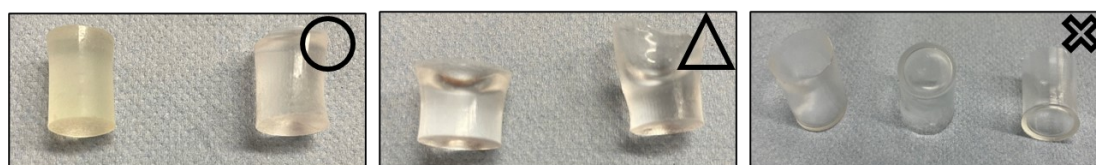
Figure 5.3 The polymer optimisation recorded for 16 batches of hybrid synthesis for different THF:GPTMS ratios, the two-pot mixing time point (mm:ss), and representative photographs of samples. The black circle represents homogeneous cylindrical shape hybrid; the black triangle irregular semi-cylindrical shape; and the black X represents formation of hollow cylinders which formed when no bubble formation occurred after added \text{BF}_3 \cdot \text{OEt}_2 catalyst in organic pot and mixed two-pot after 60 minutes. (Hybrid diameter is 1.2 cm and NA is not applicable)
