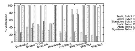
Fig.6 Precision of the P4ID 4MIDable agent using the IDS2017 traces with the BMv2 and Tofino switches
