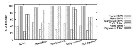
**Fig. 5** Comparison of the number of alerts and signatures raised by a Suricata IDS when using the 4MIDable P4ID agent and the ID2T trace on the BMv2 and the Tofino P4 switch frameworks
