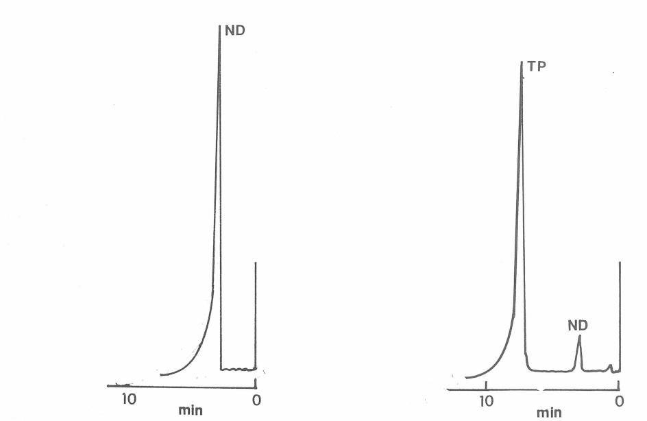
Figure 6.5 Chromatogram for sample (B). Solvent comprises acetonitrile : water (25/75) containing 20mM phosphate buffer at pH 2.0 using a 100x2mm column. Sample size equals 20ul. All peaks measured at a sensitivity of 0.05AU.
