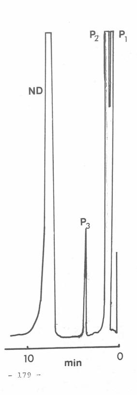
Figure 6.3 Chromatogram for sample (C). Solvent comprises acetonitrile : water (25/75) containing 40mM phosphate buffer at pH 7 using a 100x2mm column. Sample size equals 20ul. All peaks measured at a sensitivity of 0.005AU.
