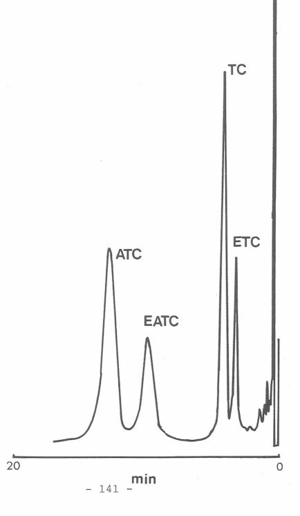
Figure 5.4 Sample chromatogram showing the separation of TC from its decomposition products using cationic pairing ion. Solvent: acetonitrile : water (40/60) containing phosphate 50mM and CTAB 2.5mM.
