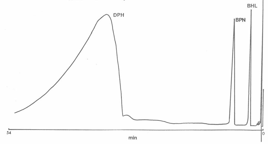
Figure 8.5 Showing the separation of DPH and its decomposition products using a 4.6x50mm column at 0.5AU. Solvent: acetonitrile : water (30/70) containing 120mM phosphate buffer, 10mM SLS and 5mM TBA at pH 2.
