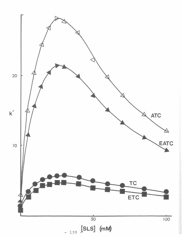
Figure 5.1 Plots showing the variation in capacity factor (k') with anionic pairing ion concentration for TC and its decomposition products. Solvent: acetonitrile : water (40/60) containing 50mM phosphate buffer at pH 2.
