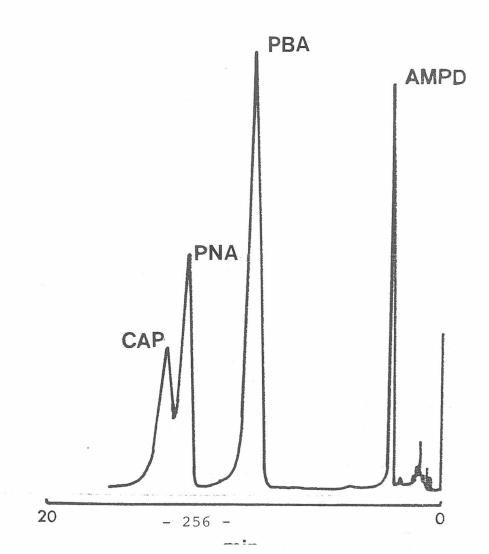
Figure 8.8 Showing an optimum specimen chromatogram for the separation of CAP and its decomposition products using a 4.6x200mm column at 0.2AU.
