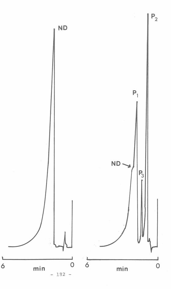
Figure 6.6 Chromatogram for sample C. Solvent comprises acetonitrile : water (25/75) containing 20mM phosphate buffer at pH 2.0. All peaks measured at a sensitivity of 0.005AU.
