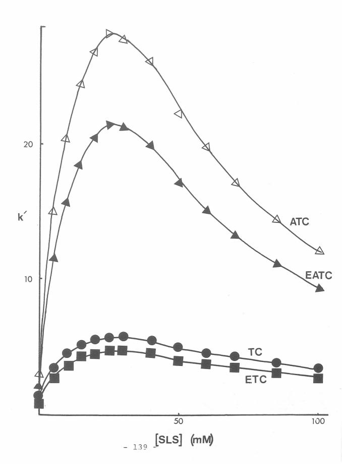
Figure 5.2 Plots showing the variation in capacity factor (k') with cationic pairing ion concentration for TC and its decomposition products. Solvent: acetonitrile : water (40/60) containing 50mM phosphate buffer at pH 7.
