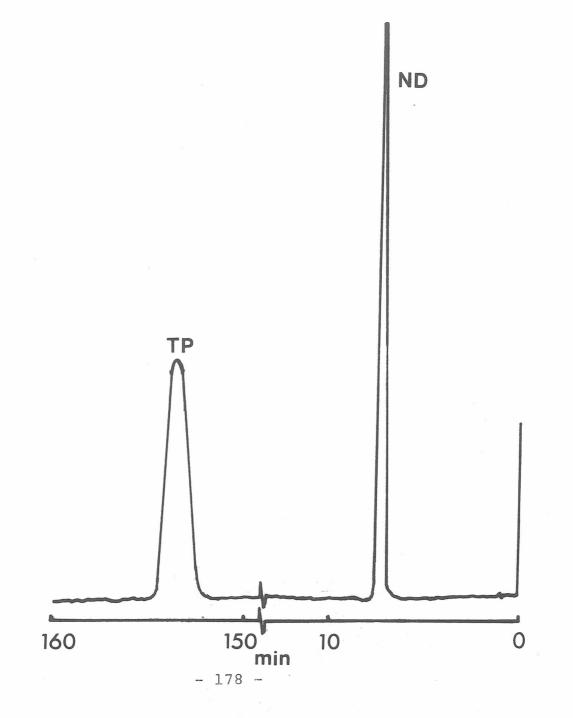
Figure 6.2 Chromatogram for sample B. Solvent: acetonitrile : water (25/75) containing 40mM phosphate buffer at pH 7 using a 100x2mm column. Sample size equals 20ul. All peaks measured at a sensitivity of 0.05AU.
