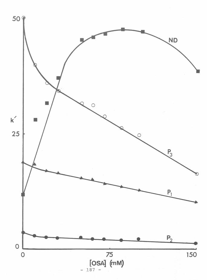
Figure 6.11 Showing the optimum chromatogram for the separation of ND and its decomposition products P<sub>1</sub>, P<sub>2</sub> and P<sub>3</sub>. Solvent: acetonitrile : water (25/75) containing 40mM phosphate buffer and 85mM OSA at pH 2.
