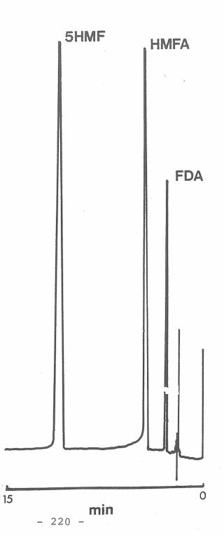
Figure 7.2 Showing the separation of 5HMF, HMFA and FDA at 0.2AU. Solvent: water containing 10mM phosphate buffer and 8mM TBA at pH 7.
