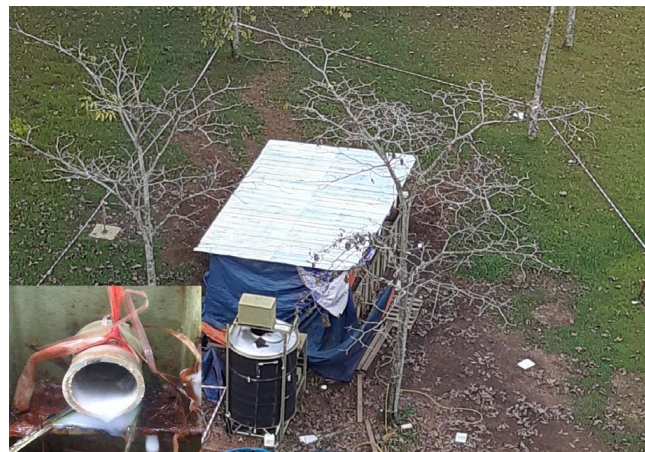
Figure 7. Leakage of ammonium-rich effluent in a 10 m 3 sandbox during an outdoor bio-cementation treatment
