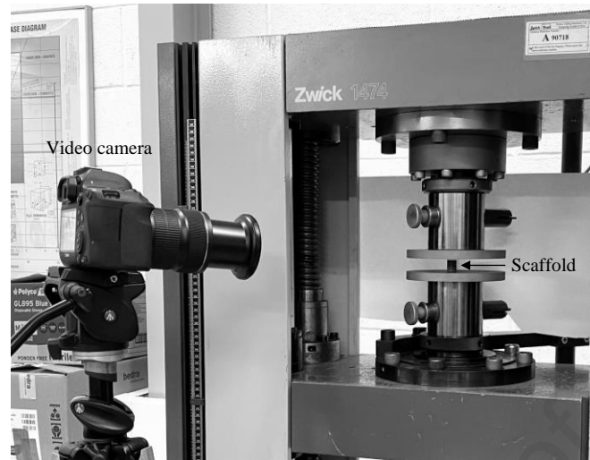
Fig. 6. Mechanical test setup showing the meta-biomaterial scaffold subject to compressive loading.
