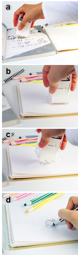
Figure 2: The Stamp-it process (a) Copy: Stamp on target image to photo capture. (b) Paste: Stamp on paper to print captured image; a cartridge moves in x-y direction. (c) Release the device after process. (d) User may edit the original image as they wish.
