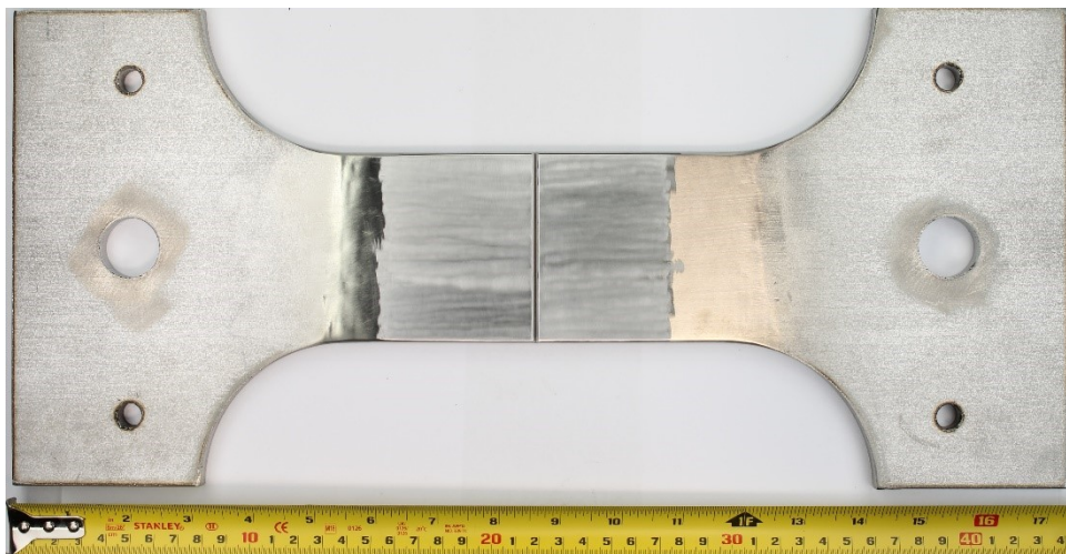
Figure 6.3–304 stainless-steel specimens for SCC tests
