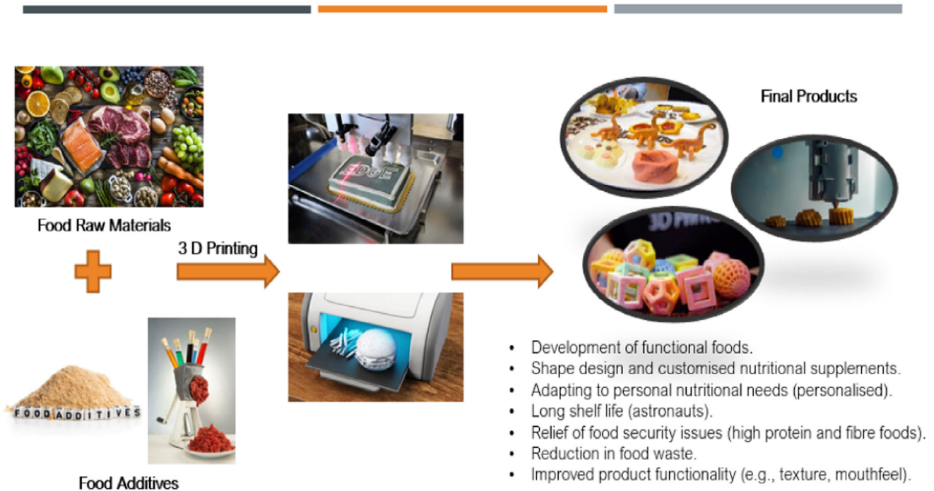
Figure 3 Principles of 3D food printing and its potential applications and advantages.
