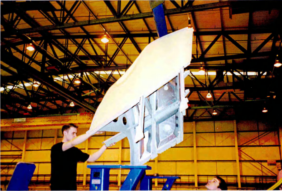
Figure 6.2.2.9 Stage 03 Build Door - Loading Bathtub assembly
