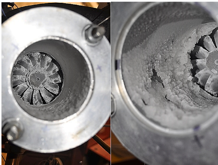
Fig. 13. Ice re-accreted in Wearlon sample during trace-wire tests.
