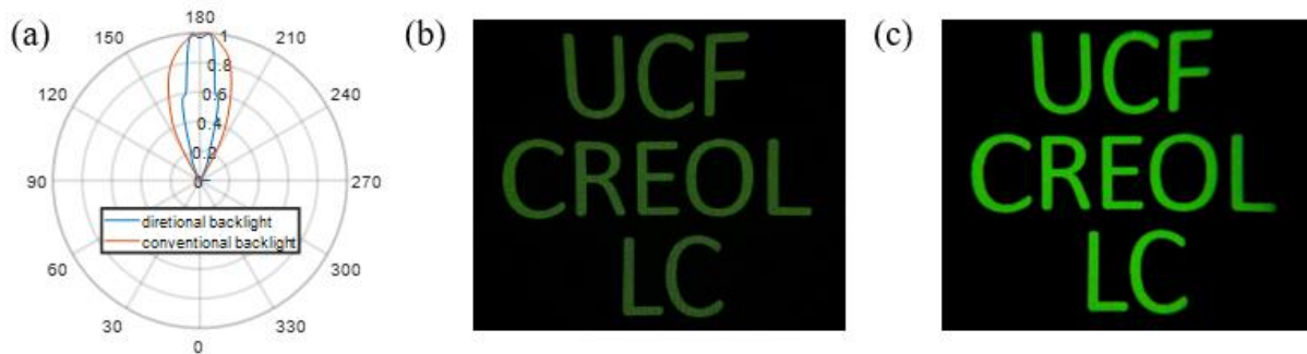
Figure 3-5: (a) Normalized angular distribution of conventional BL and directional BL. Imaging results of Fresnel system with (b) conventional BL, and (c) directional BL. The horizontal FOV of the images in (b) & (c) is around \pm 15^\circ .
