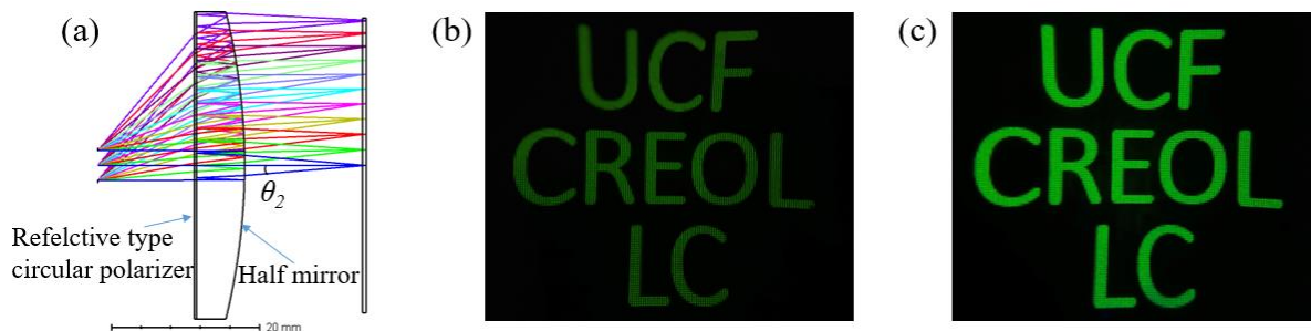
Figure 3-9: (a) Zemax profile of the “Pancake” lens. Imaging results of “Pancake” system with a (b) conventional BL and (c) directional BL. The horizontal FOV of the images in (b) and (c) is \pm 23^\circ .
