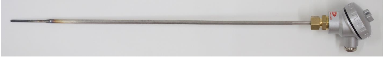
Figure 2. TC-Direct K Type thermocouple used as the steady-state temperature sensor.
