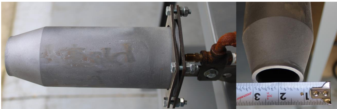
Figure 4. Ceramic burner used in testing.
