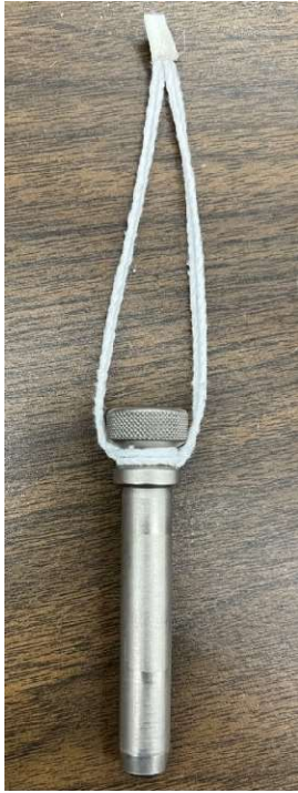
Figure 3: The impact weight measuring as 10cm long including the string, 103.87g, and radius of 12.59mm.
