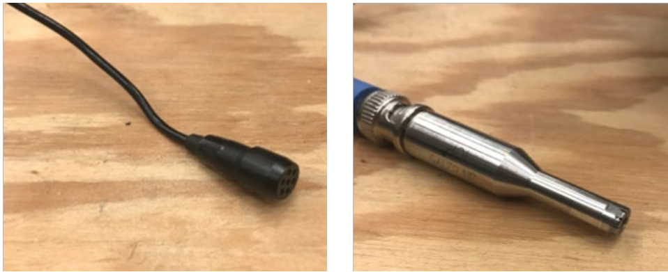
Figure 8: Lavalier microphone (left) and PCB microphone (right).
