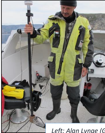
Left: Alan Lyngge (Greenland National Museum) holding the working end of the side scan system. At the lower end of the pole the transducer is shown, the upper end shows the GPS antenna. The pole is mounted on the outside of the survey vessel with the transducer being submerged in the water. Right: The transducer and GPS are connected to the top side computer unit which stores data and shows it in real time. The side scan sonar system sends out a “fan of sound” below the transducer; as the sound hits the seabed it returns to the transducer and it shown on the screen of the top side unit. A range of data can be shown in real time. (Photos: David Gregory).
