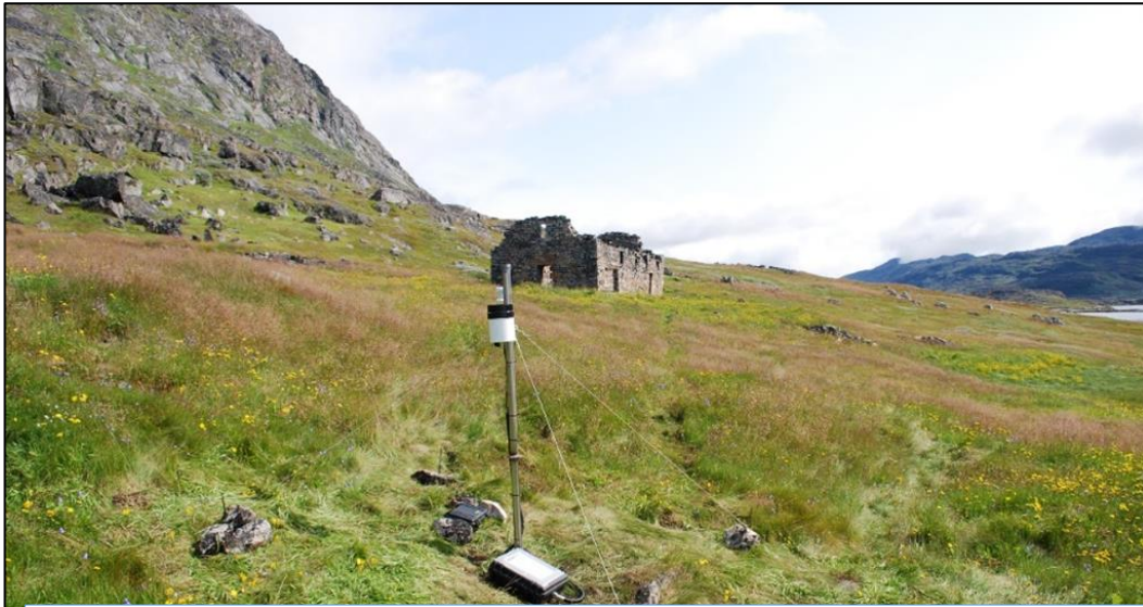
Environmental monitoring stations were installed at Hvalsey during the field campaign 2021. The station will collect time-series data on soil temperature, soil water content, air temperature and precipitation for the next couple of years. (Photo: Jørgen Hollesen).
