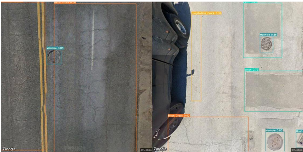
Figure 11. Segments where distress detection performed well
