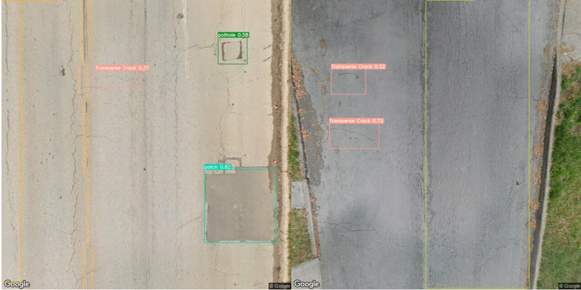
Figure 12. Segments where the model failed to detect some distresses
