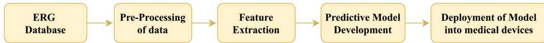
Figure 1: Machine learning workflow using ERG signals. ERG Database : the ERG database contains the input ERG data used to train the predictive model. Pre-Processing of data : this step ensures data quality by transforming the data to a common baseline, accounting for missing data, and handling outliers. Feature extraction : mathematical operations are performed on the data to extract features/parameters that indicate functional deficits in the eye. Predictive Model Development : algorithms can determine trends and patterns in data from statistical analysis of extracted features during training; these models can predict either class or value from the input data are called classifier and regression models, respectively. Deployment of Model into medical devices : successful predictive models can be included with ERG testing devices to provide real-time prognosis and diagnosis.
