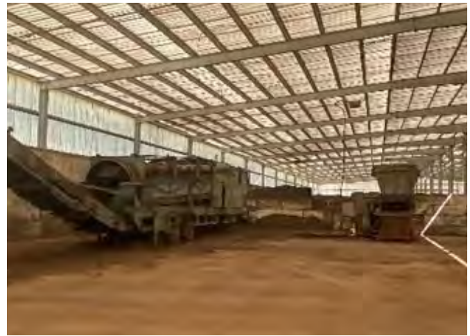
Figure 8. A compost screen was used to separate coarse woodchips and finer compost before recycling or curing.
