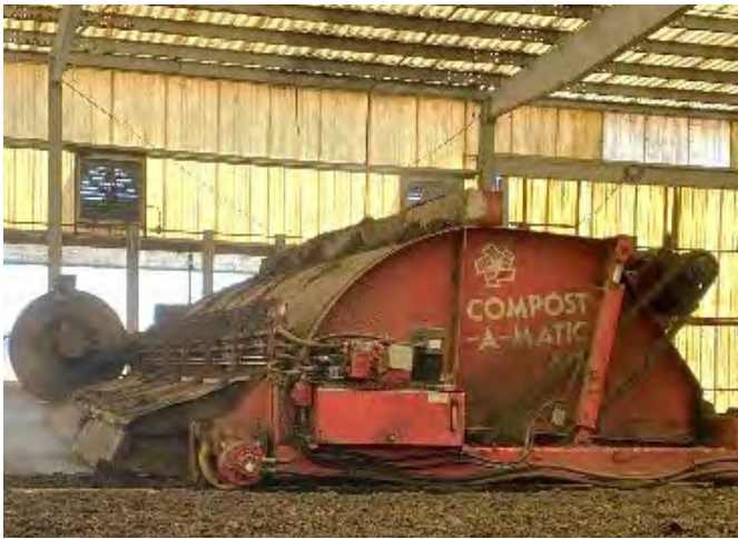
Figure 5. A mixing vessel (Compost-A-Matic 610M Agitator) working on mixing and aerating manure compost in a concrete compost pit.
