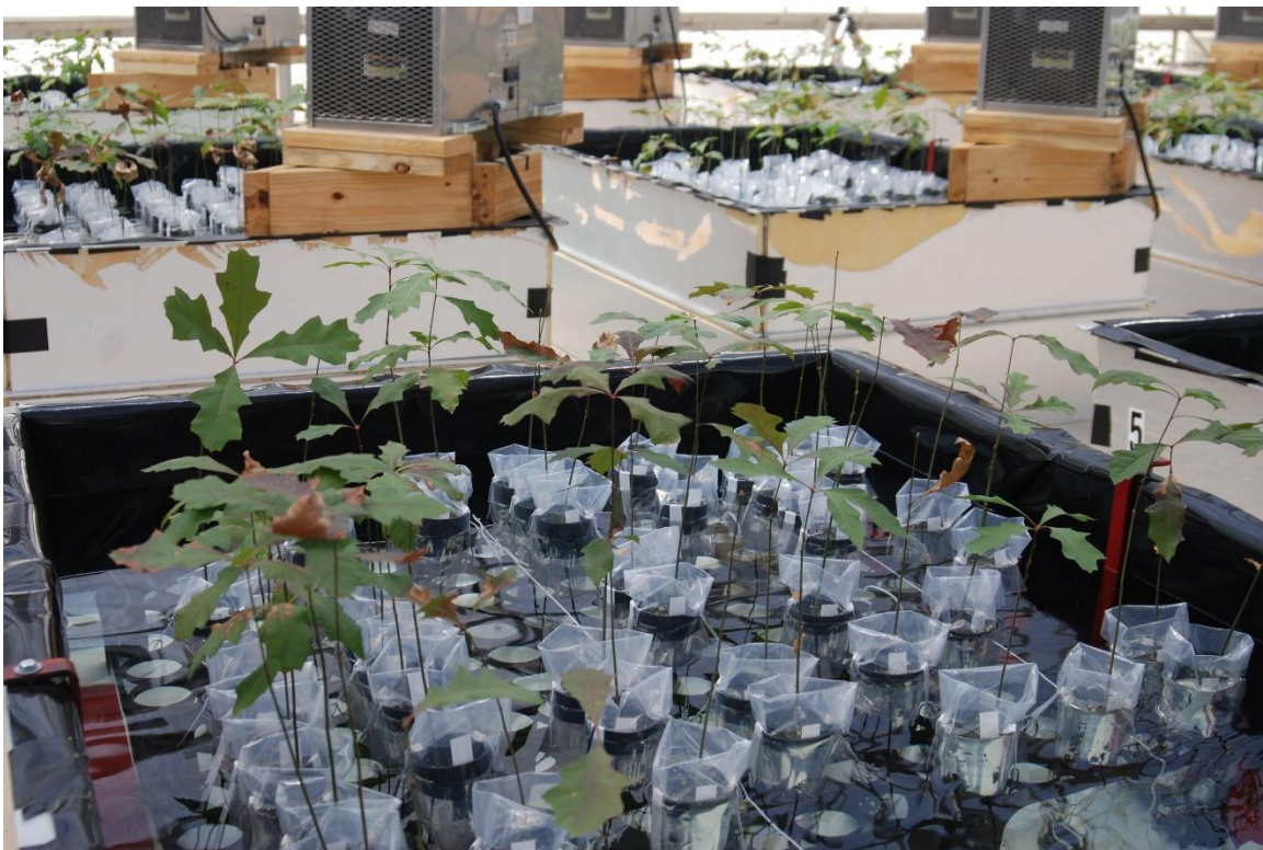
Figure 2: Photo taken March 9 of seedlings in one of the experimental water baths. The plastic bags surrounding nursery pots allow heat exchange between water and soil while preventing water from entering.
