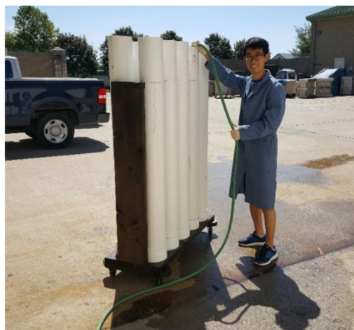
Figure 5. Use of tap water to detect leakage in reactors.
