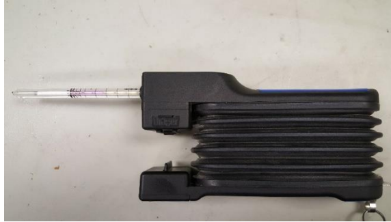
Figure 4: Hand-help below bump for detection of ammonia and hydrogen sulfide concentrations
