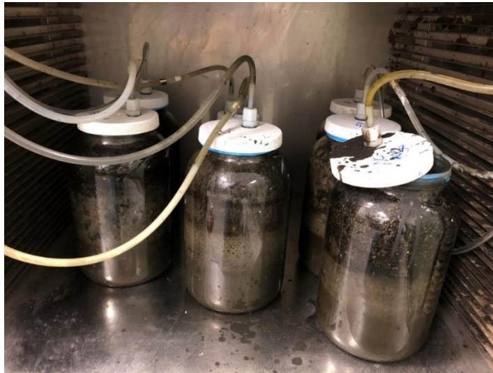
Figure 17: Explosion of biogas digester with high organic loading rate
