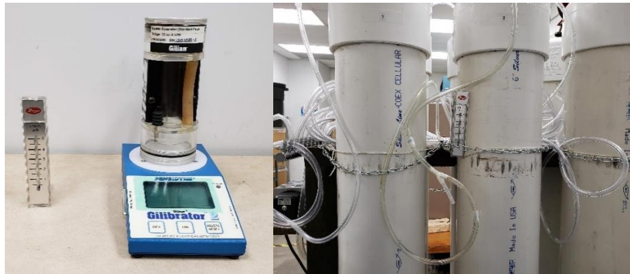
Figure 7: Airflow calibrator and rotameter for airflow measurement
