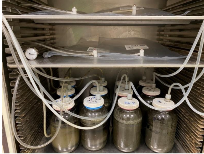
Figure 5: Set up of biogas digesters
