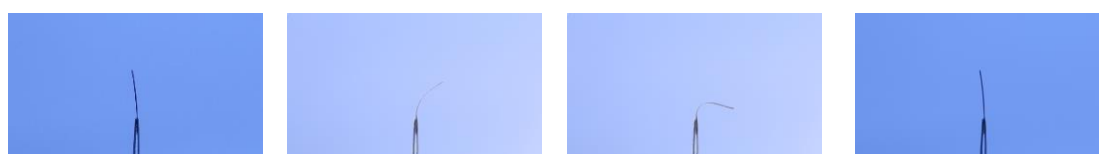
Figure 4.3.2 Optical images of the MoO 2 bending and recovering
