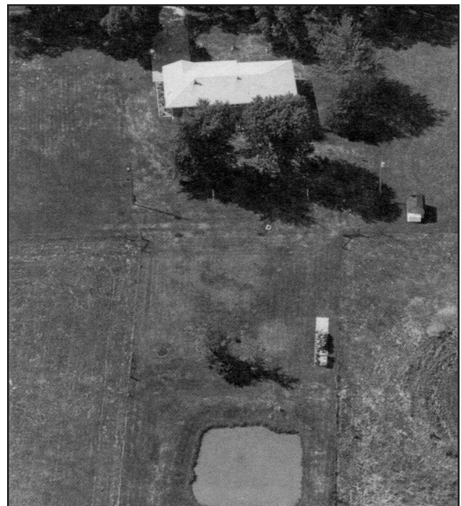
Figure 1. Aerial view of a typical residential sewage lagoon.
