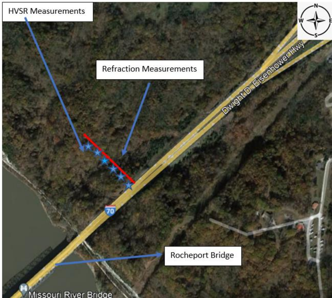
Figure 3. 11 The approximate location where six HVSR measurements were performed (star) and the refraction measurement (red solid-line).
