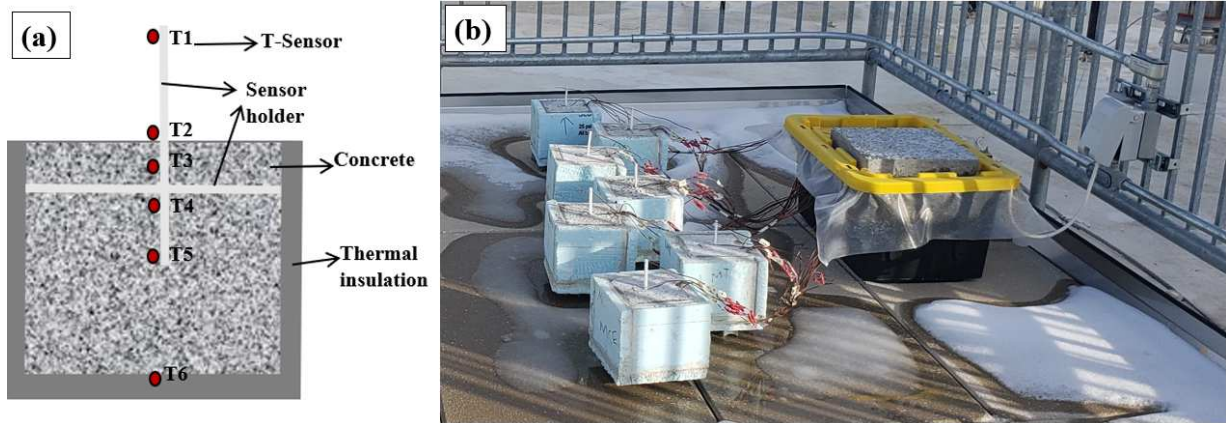
Figure 6.1: Concrete samples set-up: (a) t-wire sensors and thermal insulation, and (b) winter field tests
