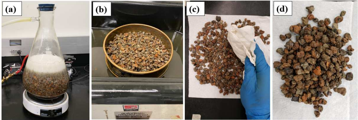
Figure 3.6: Steps for impregnating PCM into expanded clay (a) impregnation of PCM into LWA's pores, (b) drainage of PCM, (c) SSD process, and (d) TESA as final products.
