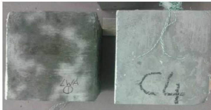
Figure 2.11: Leakage of PCM from lightweight aggregates (Niall, West et al. 2016)
