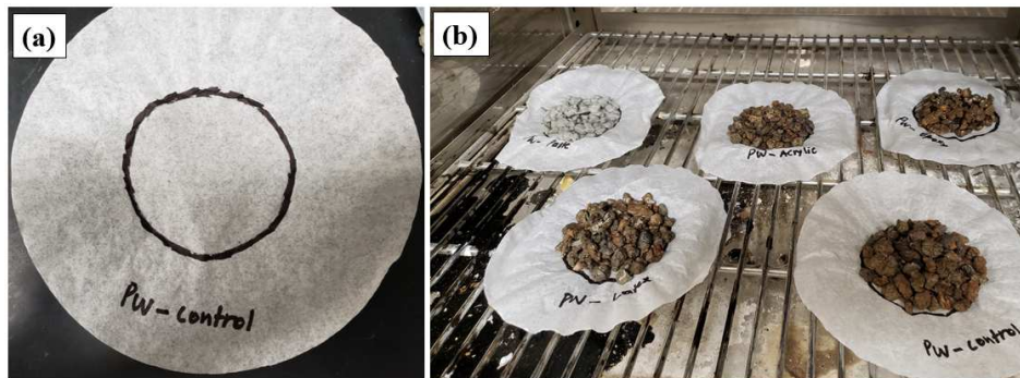
Figure 3.8: Leakage test, (a) drawn circle on a filter paper, and (b) control and coated TESA in an oven
