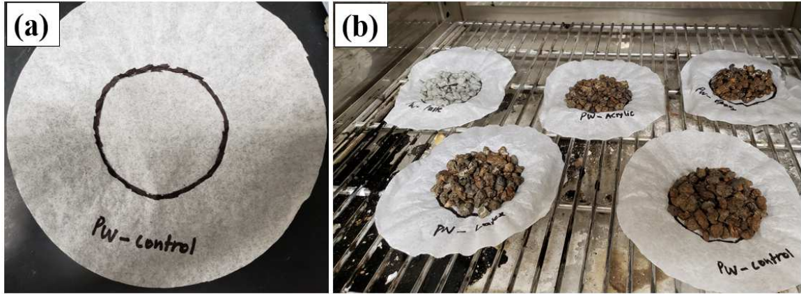
Figure 4.2: Leakage test: (a) drawn circle on a filter paper, and (b) control and coated TESA in an oven
