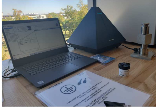
Figure 3.10: C-Therm Trident setup for thermal conductivity test of concrete cubes (50 x 50 x 50 mm 3 )
