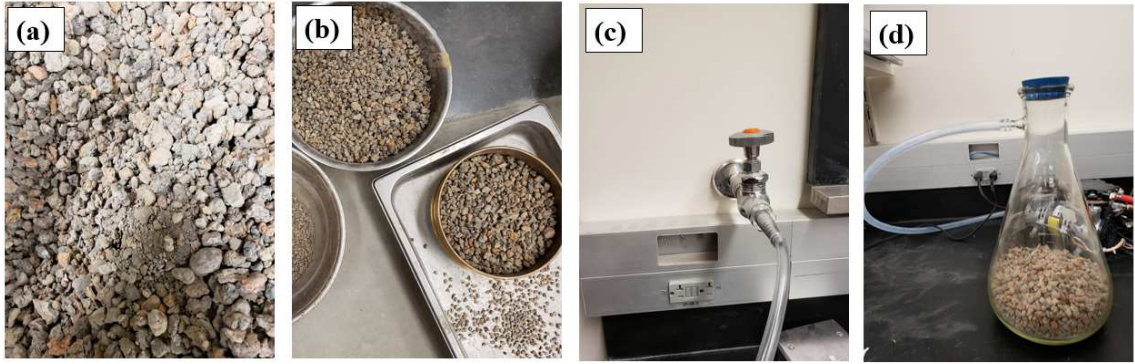
Figure 3.5: (a) As received expanded shale, (b) sieving process, (c) dusting with a compressed air, and (d) pump vacuuming of LWA
