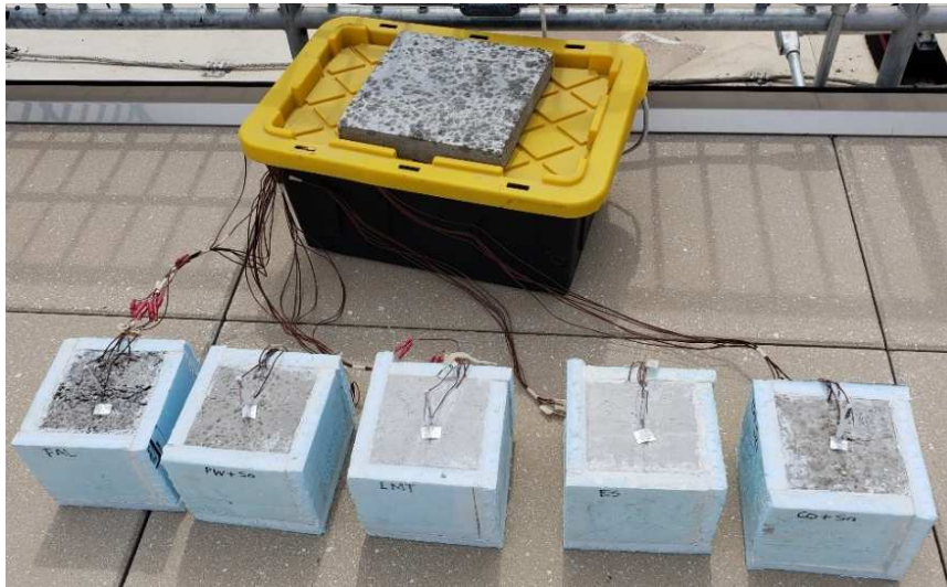
Figure 3.13: Experimental set-up of concrete cubes during summer field test
