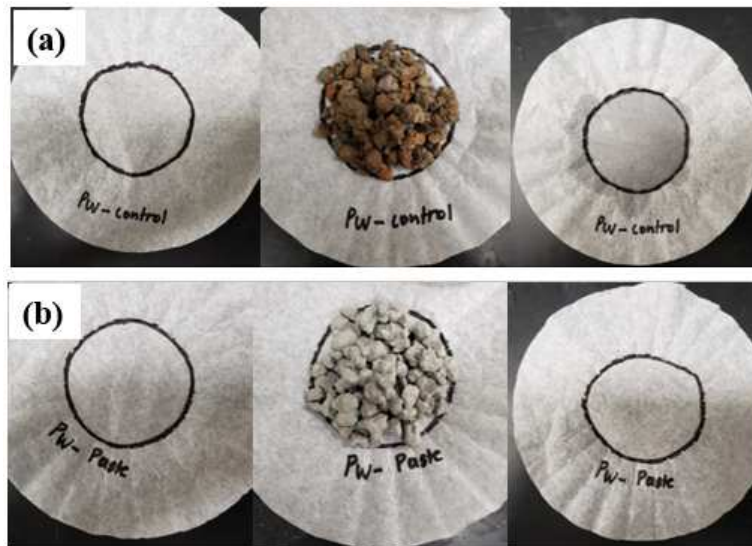
Figure 4.6: Leakage results for: (a) PW-TESA control, and (b) PW-TESA coated with the paste
