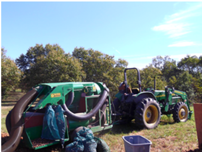
Two FACMA chestnut harvesters. BOTTOM: Tractor pulled (using PTO). TOP: Self-propelled harvester. /Photos courtesy M. Gold, UMCA.
