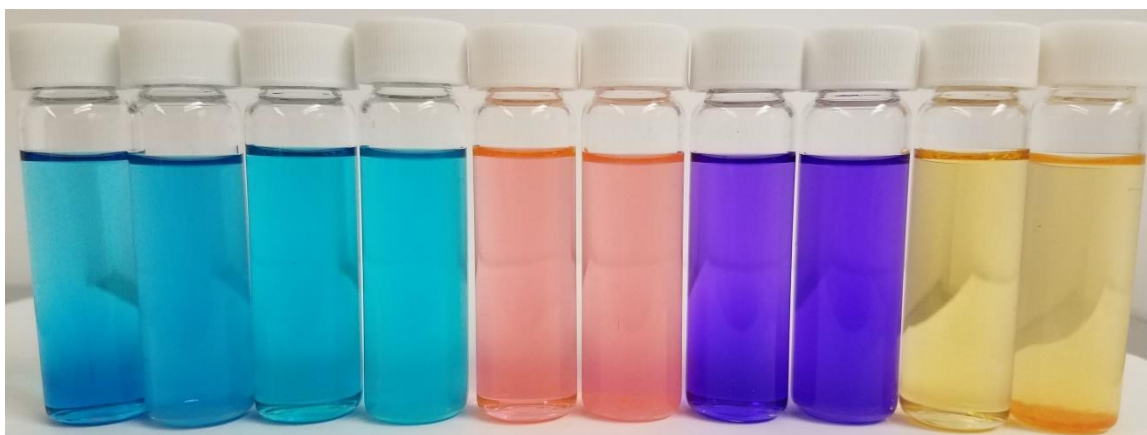
Figure 5-16: Photograph depicting the cationic dyes in acetone solutions, either in the absence of PINC (left vial) or in the presence of PINC (right vial). Dyes from left to right: Malachite Green, Methylene Blue, Phenosafranin, Crystal Violet, and Mordant Orange 1.
