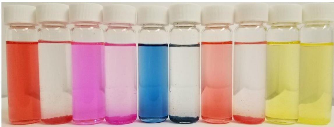
Figure 5-15: Photograph depicting the anionic dyes in acetone solutions, either in the absence of PINC (left vial) or in the presence of PINC (right vial). Dyes from left to right: Congo Red, Rose Bengal, Naphthol Blue Black, Biebrich Scarlet, and Methyl Orange.
