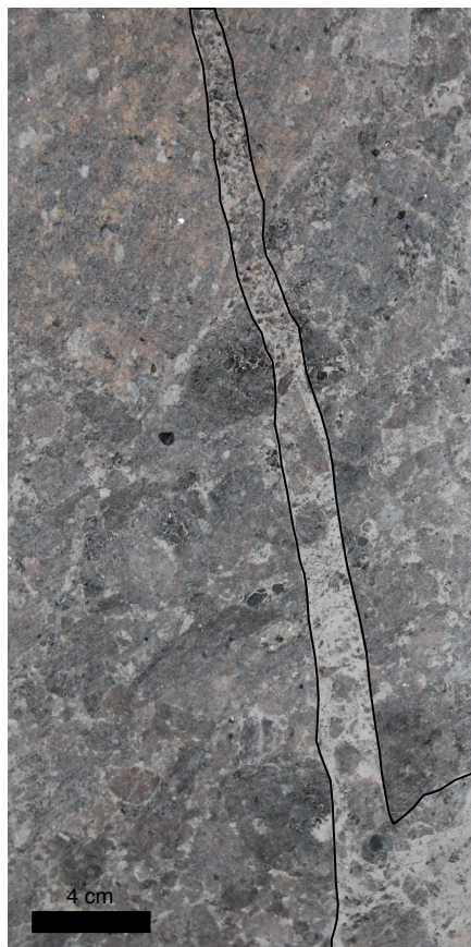
Figure 4.10 Photograph of tuffisite vein from VC-1 drill core at 490 ft (149 m) depth. Small tuffisite vein, outlined in black, cross-cutting basal breccia flow texture from Banco Bonito. Scale bar is 4 cm.
