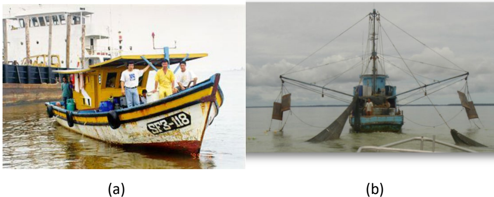
Fig. 3.3: (a) Small (40-tonnage) Zone B stern-trawler and (b) Big (70-tonnage) twin-outrigger trawler from Kuala Baram, Miri Sarawak.
