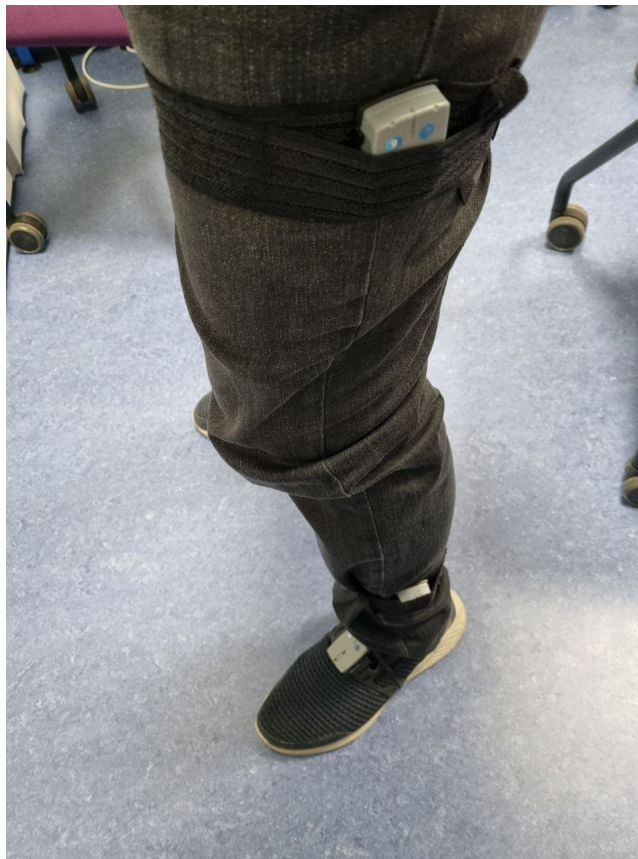
Figure B-9: IMU sensors attached to human leg
