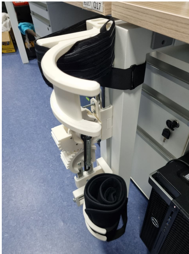
Figure B-10: IMU sensors attached to knee joint prototype
