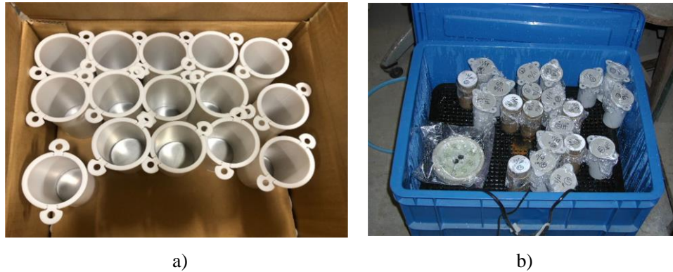
Figure 4-7 a) Plastic mold, b) Curing sample
