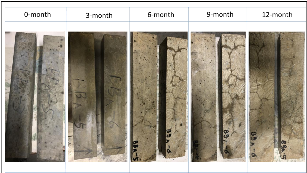
Fig. 5-3 cracks in AB-N due to ASR
