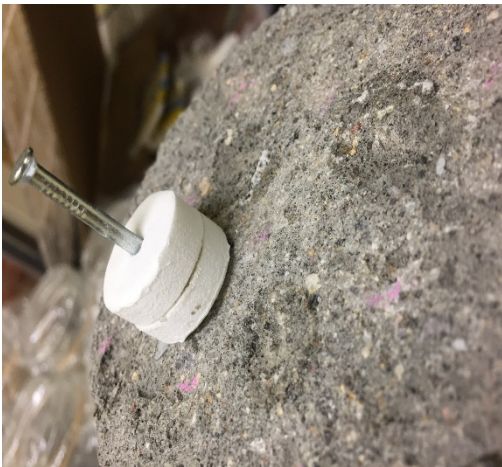
Fig. 3.9 The condition of nails fixed on the specimen
