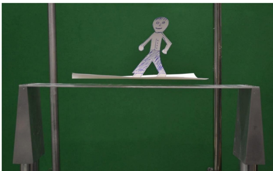
Fig.1-1.22 Acoustic levitation of a curved object weighting 2.3g [8].
