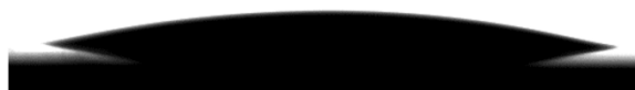
Figure S4. Contact angle image of the oil droplet on p-V 3 D 3 /Ag/TiO 2 surface.
