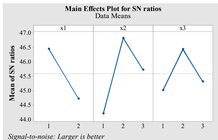
Fig. 11. The influence of the parameters on the breaking strength of the weld seam
