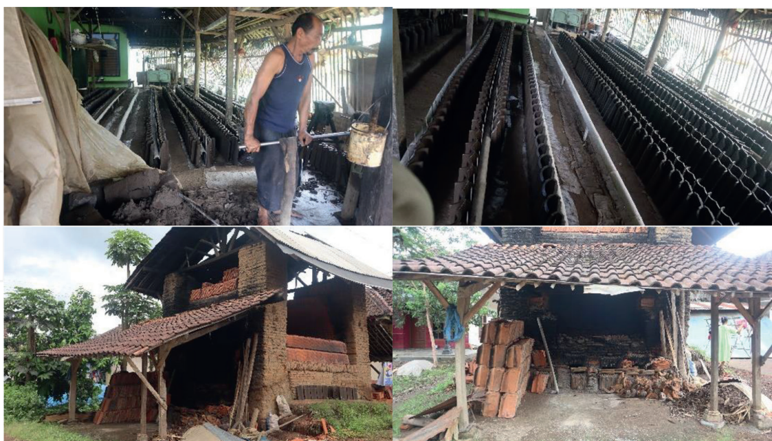
Figure 4. The production of roof tile in Urek-urek village (source: Personal documentation).
