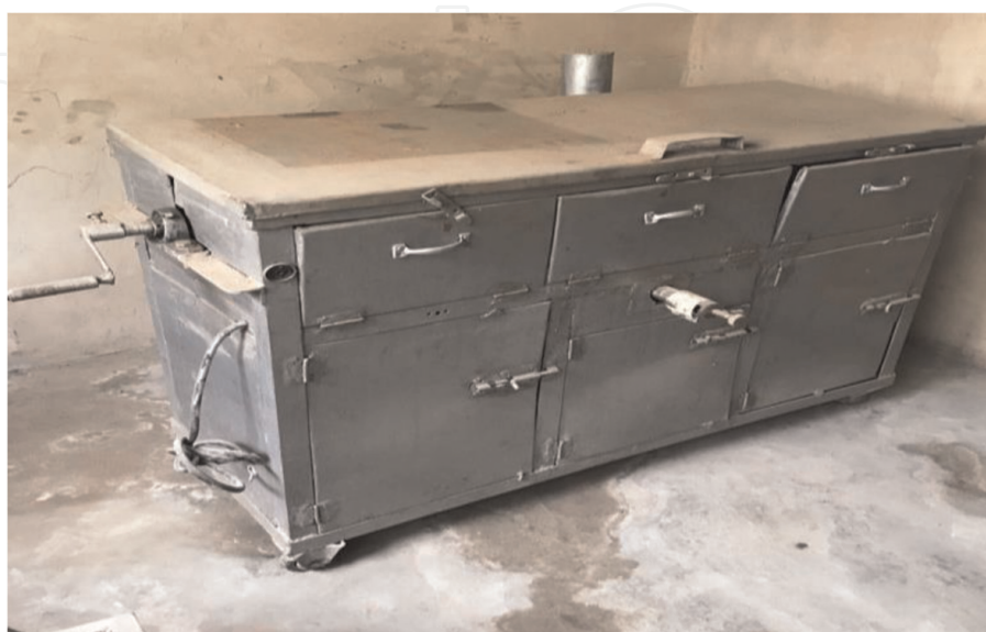
Figure 2. Snapshot of plantain roaster.
