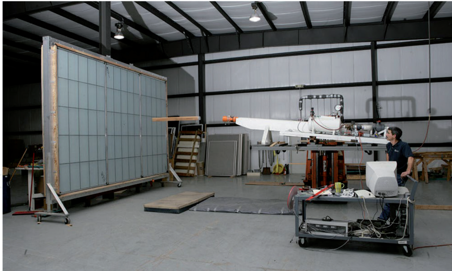
Figure 2. Impact test on a glazed façade mock-up using a large wooden missile, according to ASTM E 1886 and ASTM E 1996.
