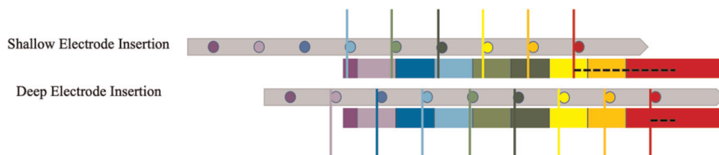
Figure 7. The effect of the degree of insertion on the magnitude of the mismatch, illustrated as dashed black line, when default frequency mapping is used.
