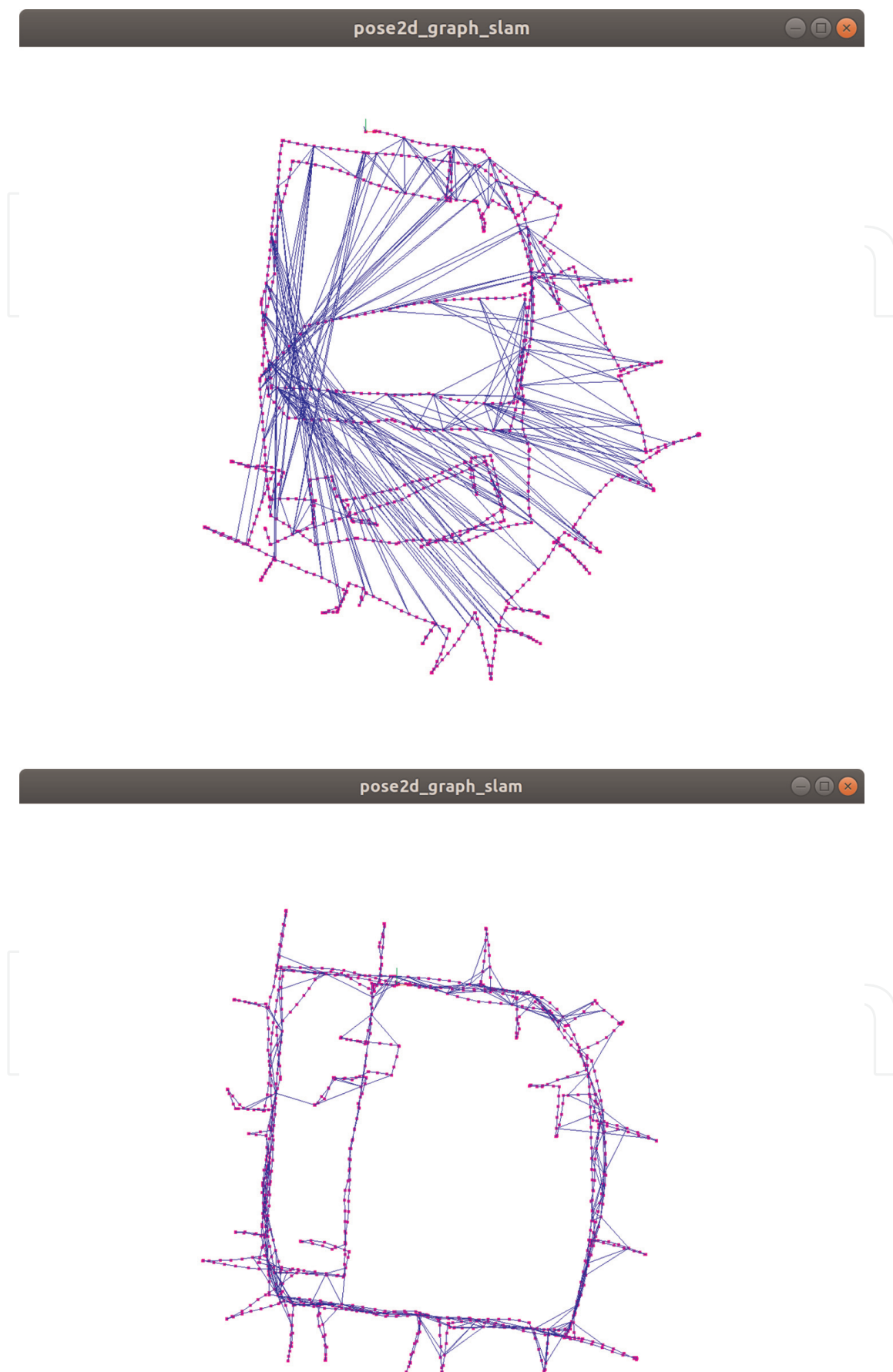
Figure 7. Top: input data for pose graph SLAM (purple dots: graph vertices, blue lines: graph edges). Bottom: result of pose graph SLAM, 2D case.
