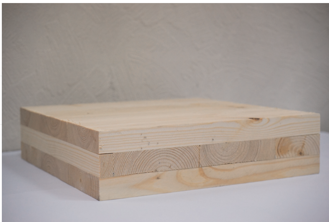
Figure 1. Isometric view of a three-layer piece of CLT construction material (Wikimedia commons contributors 2021) [4].
